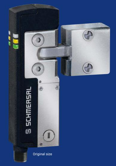
The AZM40 has a bistable interlock principle, allowing the last lock state to be retained in the event of a power failure. Even with hazardous run-on movements, the safety door remains safely interlocked.
